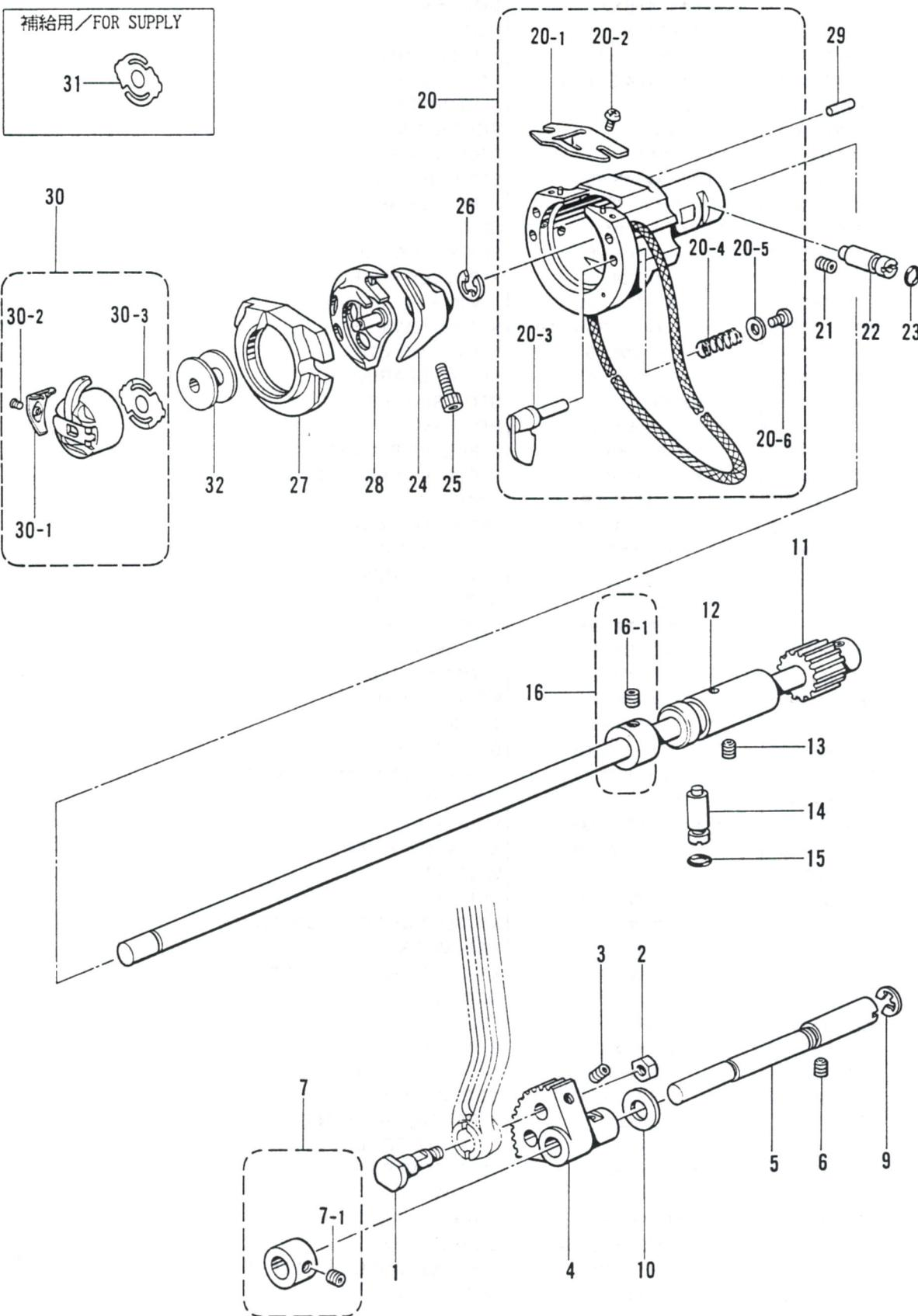
G. 下軸関係/Lower shaft mechanism/Untere Welle/
