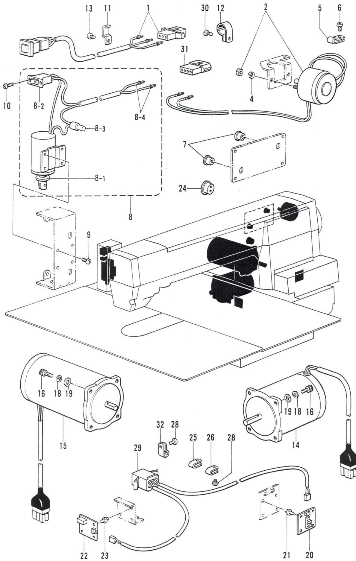
Q. 電装品関係 / Power supply equipment mechanism / Stromversorgung /
