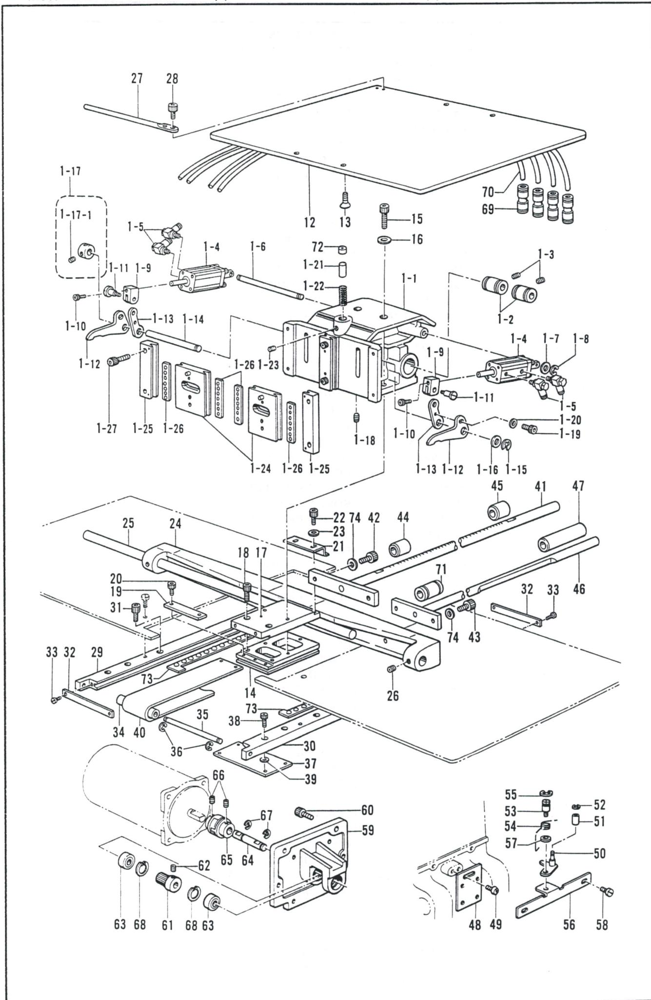
D1. 送り関係/Feed mechanism (1)/Transportvorrichtung (1)/
