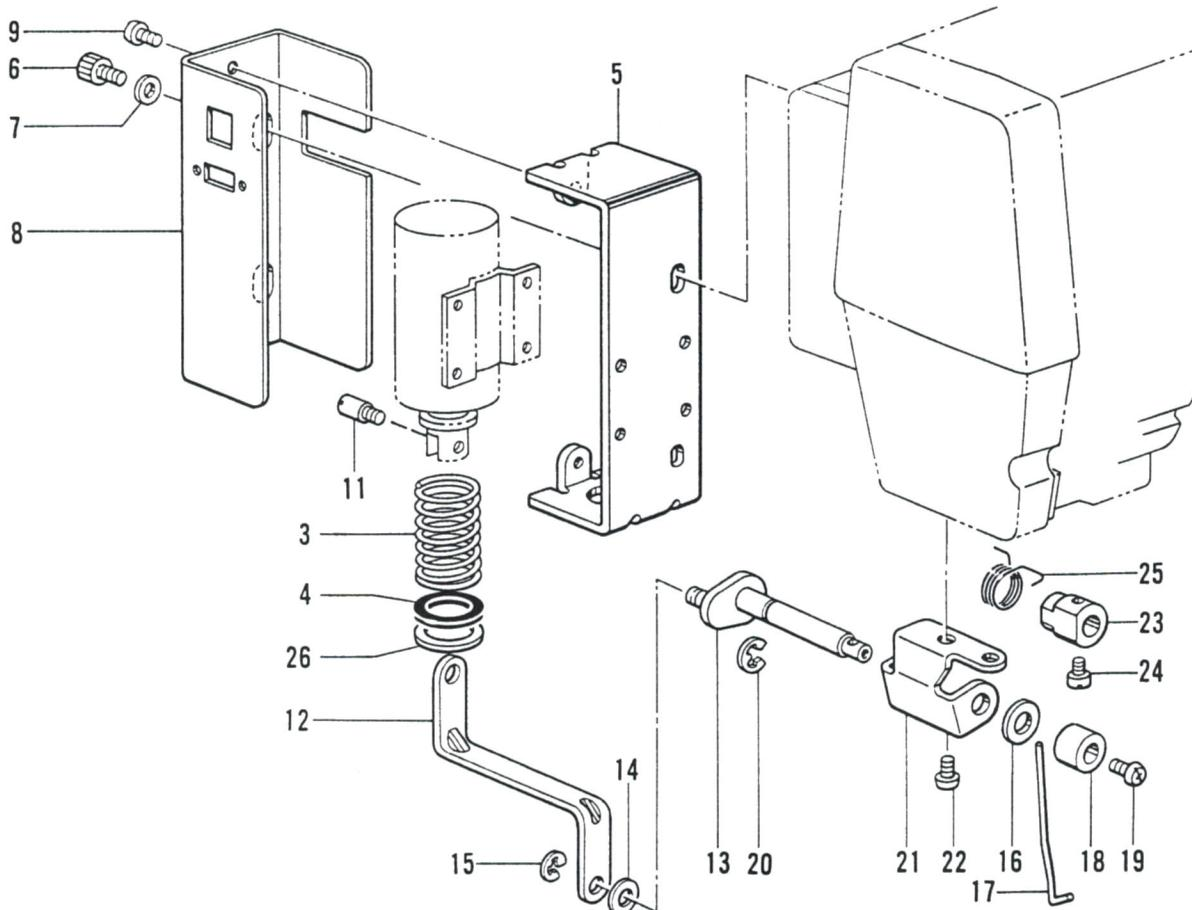
M. 糸切れ感知関係/Thread breakage detector mechanism/Fadenbruchfühler/
