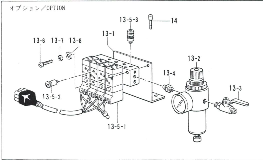
U. 空圧関係/Air pressure mechanism/Luftdruck/
